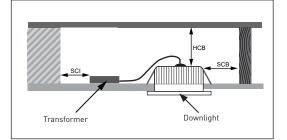
WHERE INSULATION AND BUILDING ELEMENTS ARE PRESENT: (SCB = HCB = SCI = 50 mm minimum)
